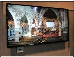
High definition camera images with audio is relayed to the crèche LED monitor. A local HDMi input allows the display to be utilised for independent meetings.
